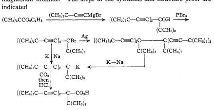
This ethane was found to be more stable than the corresponding diphenyl derivative (II) since cleavage could be accomplished only by use of liquid sodium-potassium alloy. The ethane was stable toward heat at  $140^{\circ}$ , since it could be recovered unchanged after boiling the xylene solution. It did not absorb oxygen when dissolved in *p*-dibromobenzene and heated to  $140^{\circ}$ .
